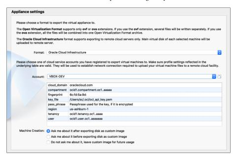
In the **Machine Creation** field, select an option to configure settings for a cloud instance created when you export to Oracle Cloud Infrastructure. The options enable you to do one of the following:
